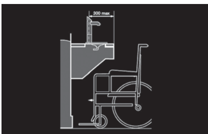
Font installation to accommodate disabled access.
